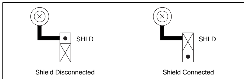
Figure 10-4. Ground Settings for Jumper W1
